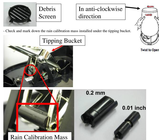
The larger and smaller weight is for measurement in 0.2 mm and 0.01 inch for each flip of the tipping buckets. Settings in WeatherLink and console mismatch with the actual installed mass would give underestimated/overestimated amount of precipitation.
