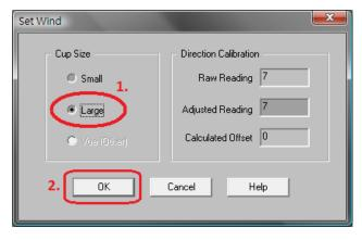
If the anemometer mounting bar cannot be set to pointing north, please input the current direction in degree in "Adjusted Reading" to amend the wind direction.
