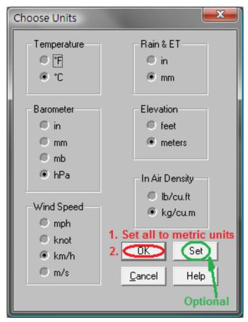
If you also want to set units display on console by WeatherLink, press "Set" (may require to reboot the console by disconnecting all power sources (A/C adapter and batteries)).
